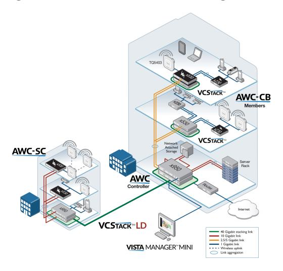
Allied Telesis Autonomous Wave Controller (AWC) offers solutions for two of the most common problems with Wireless LANs: initial setup complexity and on-going performance degradation. Initial WLAN set-up usually requires a site survey to achieve the best coverage; and performance of WLANs can often change over time as external sources of radio interference reduce coverage and bandwidth. These issues can be time-consuming to identify and resolve.
