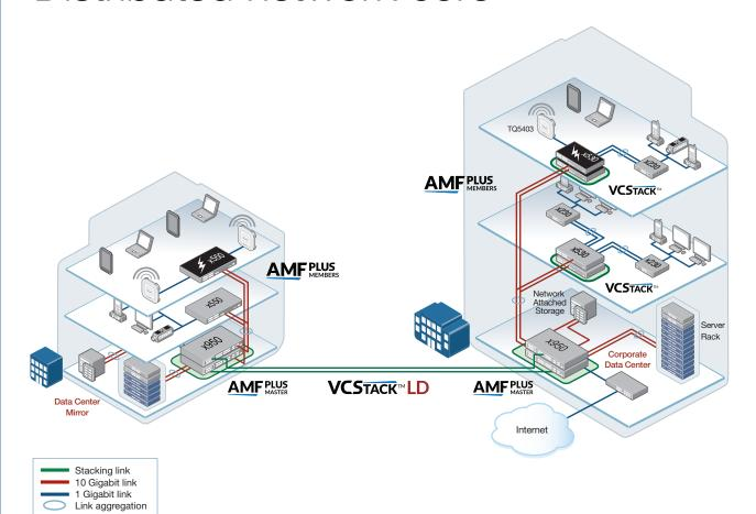
Today's corporate network users demand a high-performing enterprise network that can seamlessly carry multiple converged services, and provide instant access to online resources and applications. This key solution uses the x950 Series and VCStack LD—ideal for a distributed business network core that provides high
